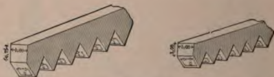
FIGS. 165-166.—SHEET-IRON FLUES WITH TRIANGULAR PROJECTIONS.
